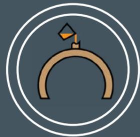
Molten steel alloy is poured into the ceramic shell and left to set.
