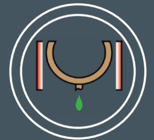
Wax is melted and pulled away, leaving just the ceramic shell behind.
